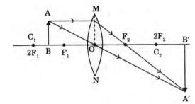
When object is placed in between  $F_1$  and optical centre O of a converging lens, it will form a virtual magnified image of the object.
