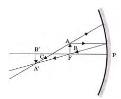
**55.** Discuss the position and nature of the image formed by a concave mirror when the object is moved from infinity towards the pole of the mirror.
