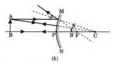
Convex mirrors are used in automobiles as a rear view mirror because of wider field of view and formation of erect image.
